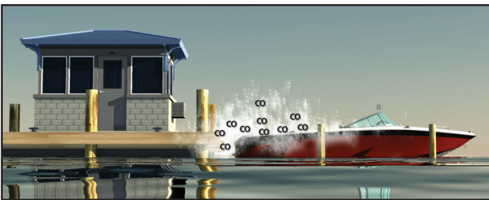
Blockage of boat exhaust by obstruction.
