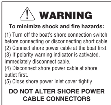
Shore Power Connection
