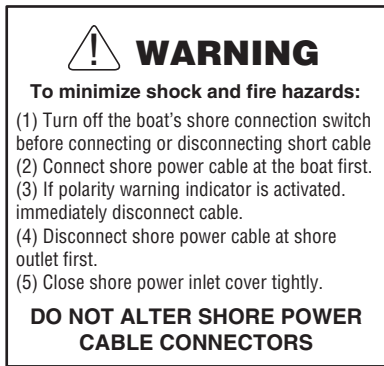
Shore Power Connection
