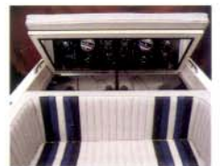
Electric powered hatch gives easy access to engine compartments on the Condurre series.
