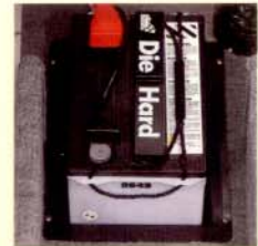
Recessed battery box for superior battery stability.
