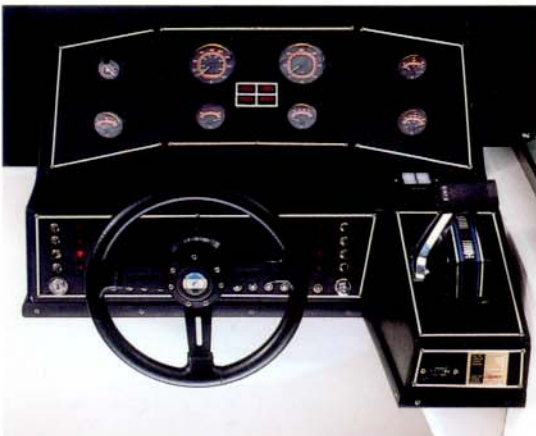
Flat black, aluminum glare-proof dash panel with full instrumentation featured on the Corista.
