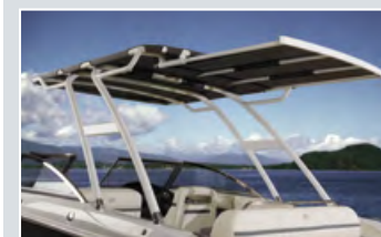
A permanent rigid structure with a stretched canvas top covering, and the extendable sunshade aft. Available for models 23SC and 25SC.
