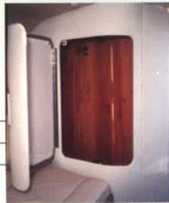
Cedar Lined Locker
